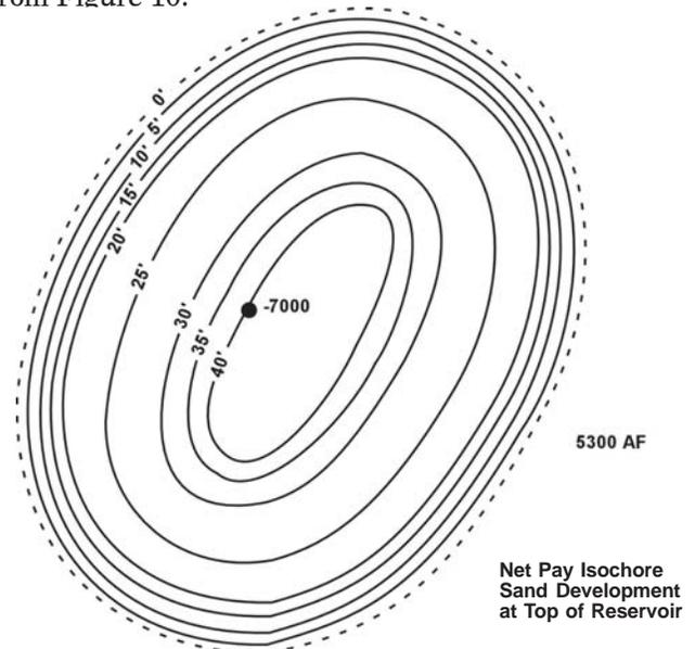
Figure 10. Same data mapped with wedge zone based on correct application of a vertical net-to-gross ratio.
